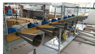
Calibration - radar level transmitters
